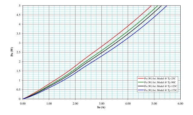
FIGURE 12. Rectifier power versus I<sub>0</sub> (average forward current) for 1N5807(US), 1N5809(US), 1N5811(US).
