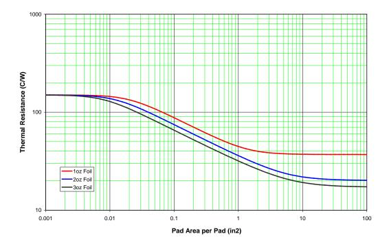
FIGURE 13. Thermal resistance versus pad area still air, PCB horizontal, (for each pad) with 1, 2, and 3 oz copper for 1N5807(US), 1N5809(US), 1N5811(US).
