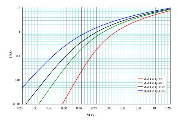
FIGURE 17. Forward voltage versus forward current for 1N5802(US), 1N5804(US), 1N5806(US).
