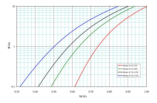
FIGURE 14. Forward voltage versus forward current for 1N5807(US), 1N5809(US), 1N5811(US).
