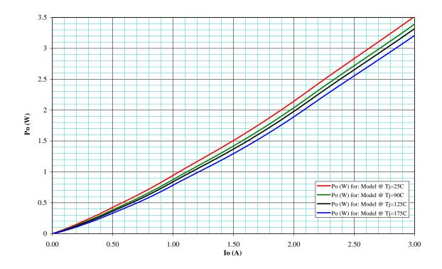
FIGURE 15. Rectifier power versus I<sub>0</sub> (average forward current) for 1N5802(US), 1N5804(US), 1N5806(US).
