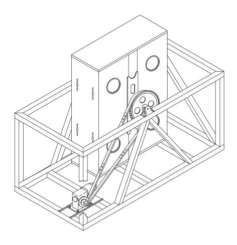
FIGURE 1. Typical assembly of four-cage random-drop-test machine.
