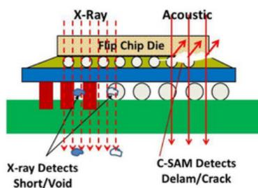
**Figure 1.** X-ray vs Acoustic Microscopy reprinted from "ECS Transactions, 33 (4) 47-57 (2010)"
