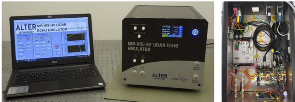
Fig. 11. The realization of the LEE: hardware and software (left) and the top level inside NIR-VIS-UV LEE (right).
