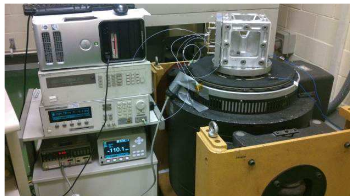
Fig. 13: Vibration Test Setup
