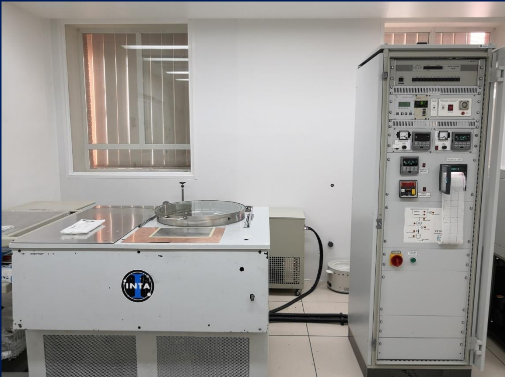
MODEL DMAVAC –Horizontal heating –cooling plates Developped by INTA
